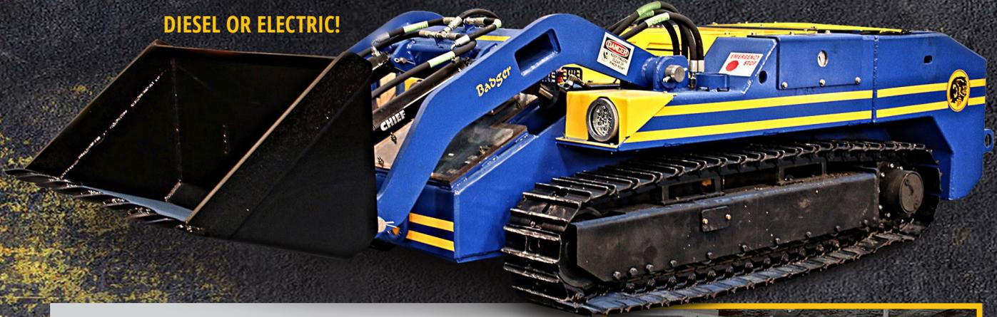
The GMS electric- or diesel-powered Badger is a robust, remote-operated, excavation and utility machine, that is nimble and compact enough to access areas too precarious or difficult to reach for a traditional skid steer or dozer. Underground examples include excavation in narrow or low areas, and under conveyors. Above ground, typical uses include highwall bench cleaning and remediation, or culvert and confined space cleaning.
